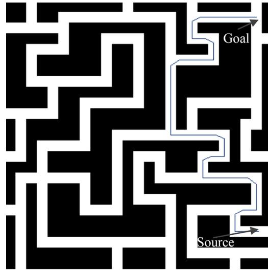
Figure 10(b): Path traced by robot 2 for simulation with 5 robots
