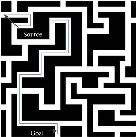
Figure 10(a): Path traced by robot 1 for simulation with 5 robots
