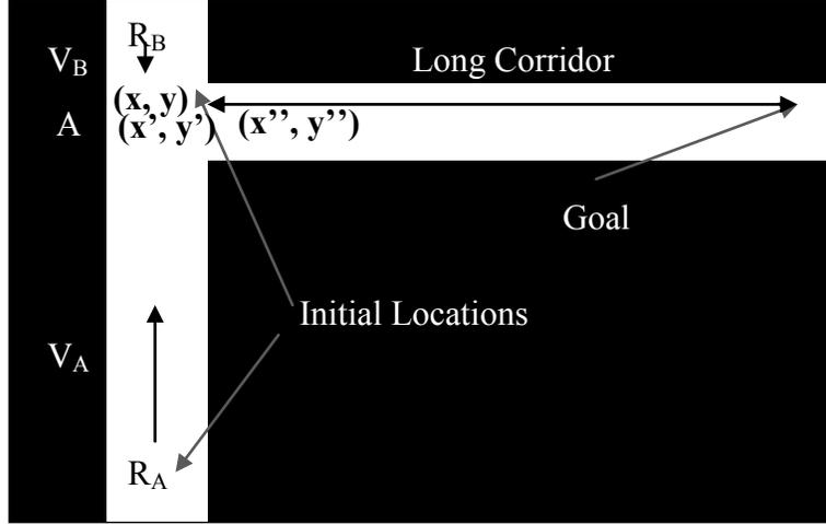
**Figure 6: The problems with planning with multiple speeds.** The figure shows two robots  $R_A$  and  $R_B$  moving with velocities  $V_A$  and  $V_B$  ( $V_A \gg V_B$ ). If  $R_B$  enters the corridor first,  $R_A$  will have to follow for the rest part of the journey with reduced speeds. Optimal path has  $R_A$  entering before  $R_B$ .
