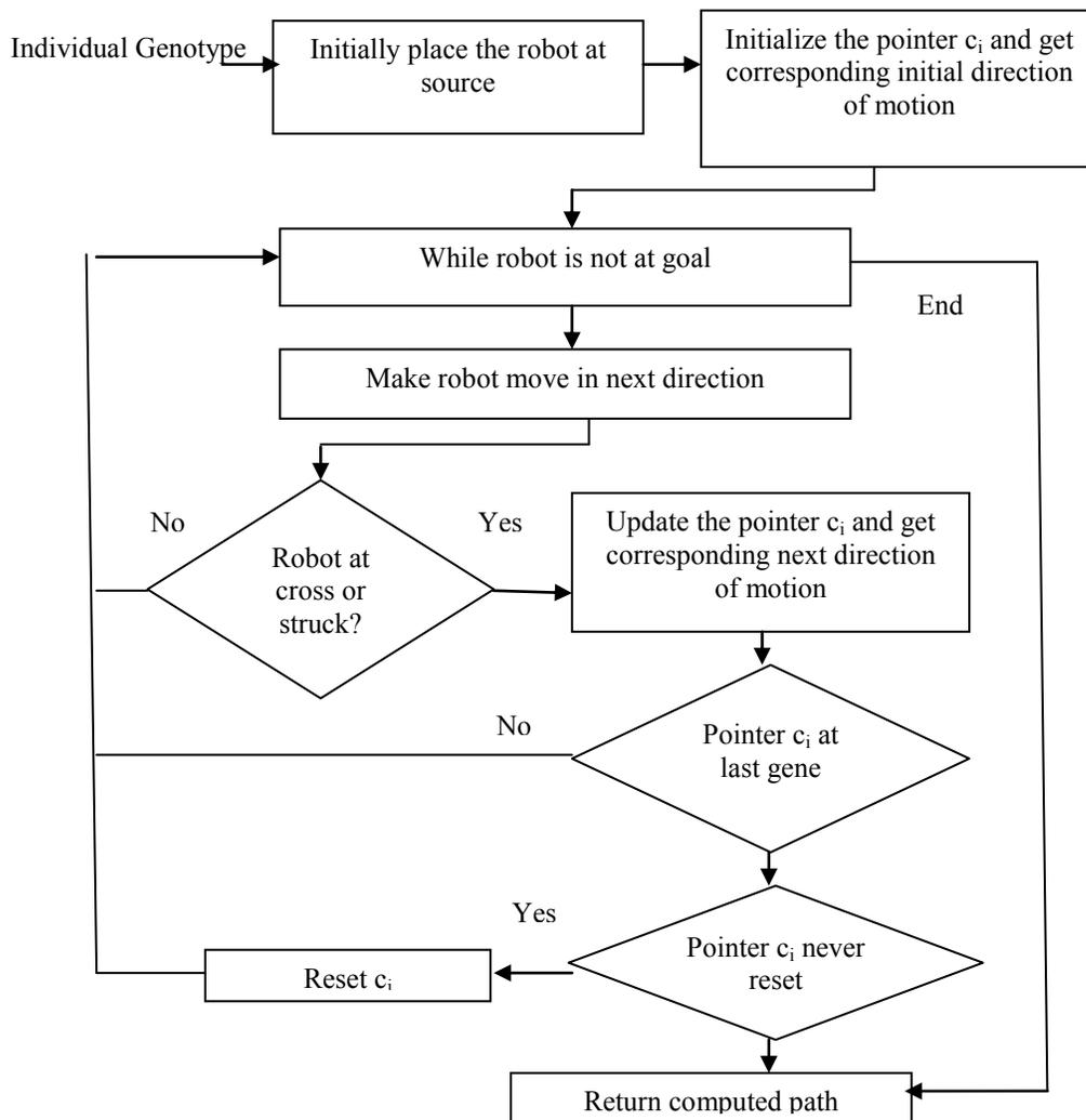
**Figure 2: Conversion of a genetic programming genotype to robotic path phenotype.** The algorithm takes an individual which is a collection of integers. The robot is moved in its computed direction. Whenever any cross is encountered, the pointed integer is consulted to get the next direction of motion, and the pointer is updated. The algorithm terminates if goal is found or when the individual terminates twice.
