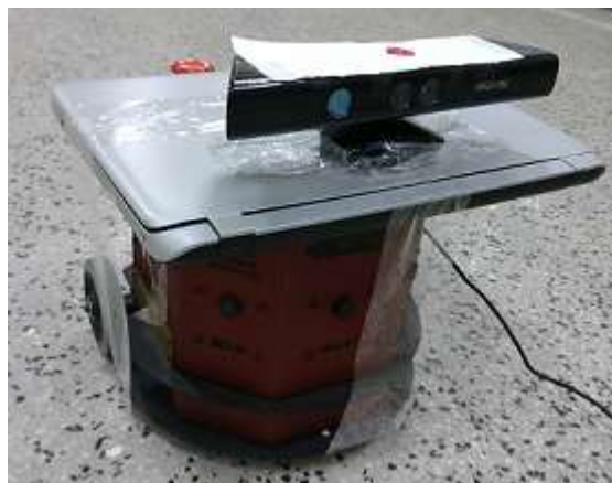
Figure. 7: Robot Platform Used for Experiment: The Kinect has been attached to a Firebird 6 robot.
