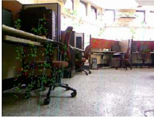
Figure 2: GFTT Features: The green dots show the GFTT feature points detected in our image.
