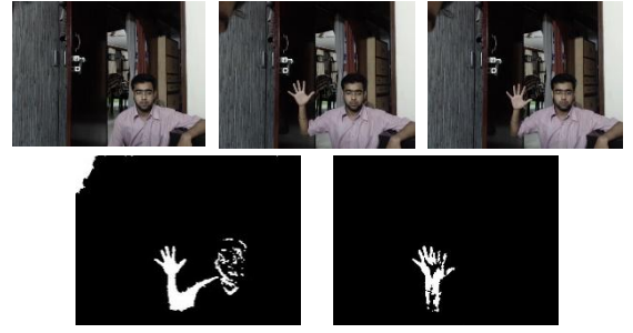
Fig. 1. a) The background frame F(0) , b) A regular frame F(n) , c) The previous regular frame F(n-1) , d) Final result of background subtraction, e) Final result of sequential frames subtraction.
